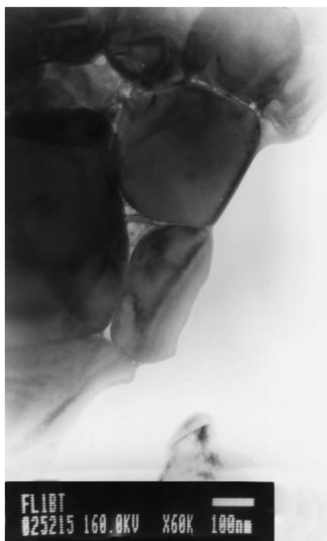
FIG. 8. Bright field TEM micrograph of flux (1) sample sintered at 1000°C showing second phase at grain corner and along the boundary.
